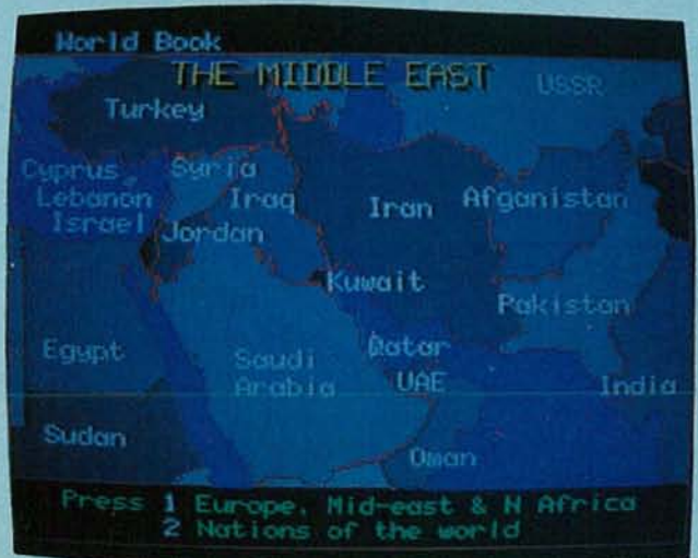
FIG. 4—TELIDON ALLOWS shapes and special character-sets to be defined and then recalled by a single command.
